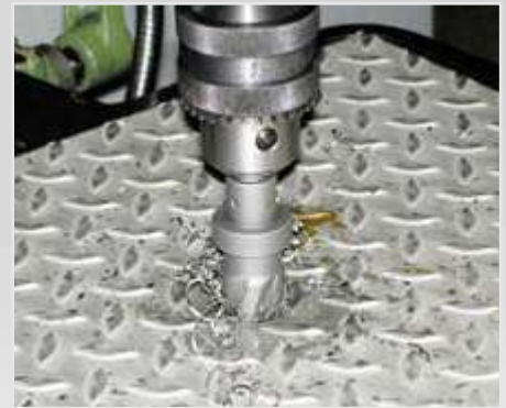
Drilling structured sheet metals
