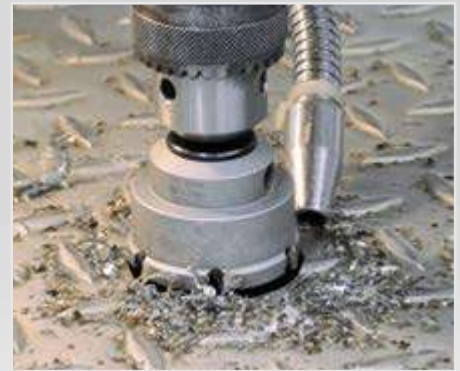
Drilling in checker sheet
