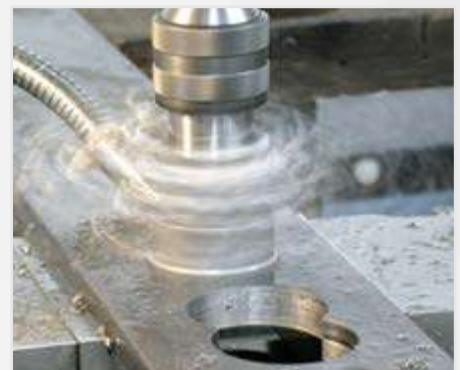
Drilling in flat steel
