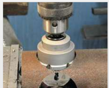
Drilling in pipes
