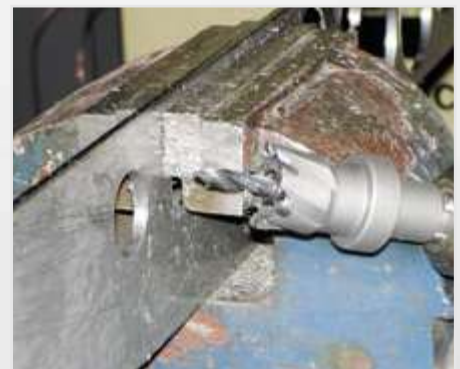
Free-hand drilling up to Ø 30 mm
